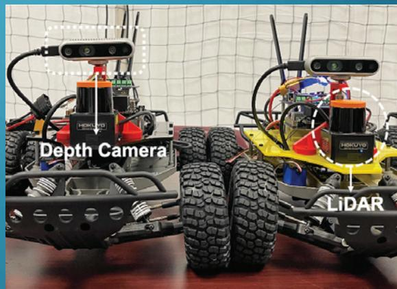
The physical cars used in the testbed and the two major sensors used in self-driving technology.
