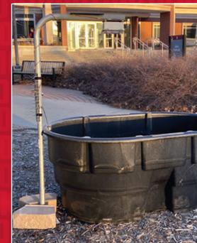
A CK Monitor Test Device runs on a testing tank on campus for environmental testing and website coupling testing.
