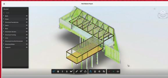
ZeroDelta's custom viewer built on Autodesk Platform Services displaying the comparison model classifying points that correspond to 3D model.
